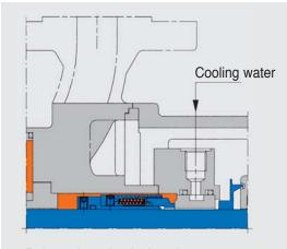
Balanced mechanical seal, stationary seat with cooling jacket
