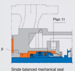
single balanced mechanical seal p > 10 bar
