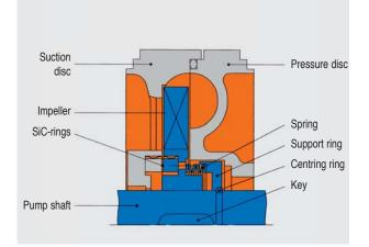
The SiC-rings are placed in the suction and pressure disc as well as in the impeller hub. The impeller ring will be pushed concentric to the ring in the disc by the spring and the support ring. Metallic contact between the rotating and stationary parts and seizing of the impeller are excluded.
