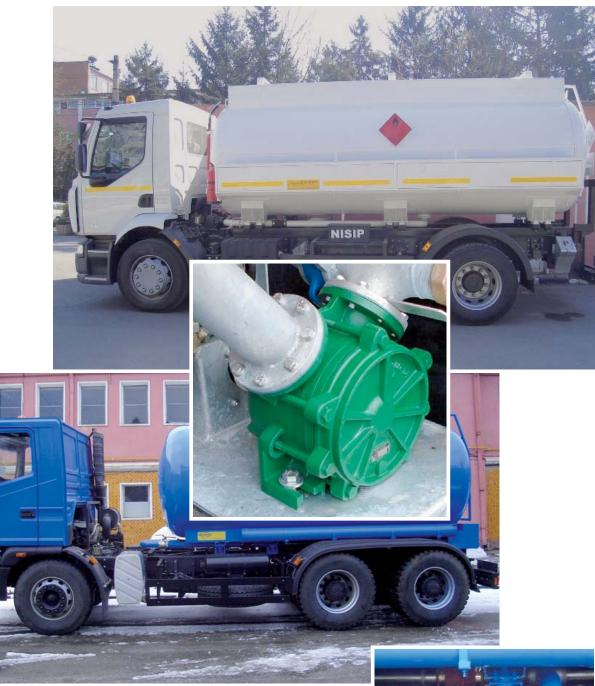
Self Priming Side Channel Pump Tank Truck Execution
