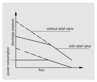
Contrary to centrifugal pumps, the side channel pumps generate a steep head rise and an increased power consumption at lower flow rates. Power consumption and discharge pressure reach the maximum at closed discharge valve. To protect discharge pipes and to avoid overload of the motors, additional relief valves can be fitted to the WPC-pumps.
