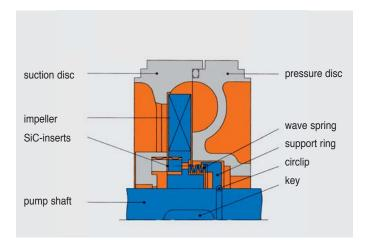
To increase availability and to avoid seizing of the impellers in any case, the pumps can be fitted with additional SiC-rings as an option.
