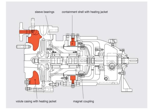
Type NMR o - with open impeller and edge type filter
